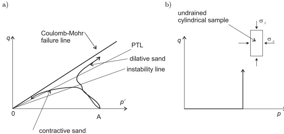
FIG. 1. a) Effective stress paths followed during the undrained shearing of saturated sand.
