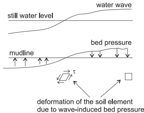
FIG. 9. Bed pressures caused by water waves and the resultant cyclic deformations of the seabed.
