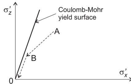
FIG. 13. The effective stress path followed during an increase in pore-pressure, under constant total stresses.
