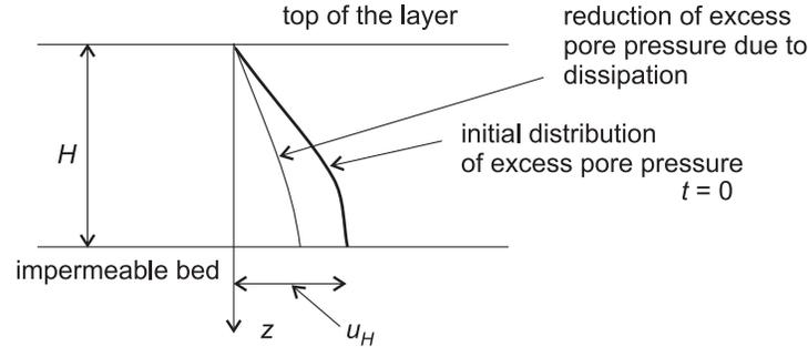
FIG. 6. Example of pore pressure dissipation in a saturated soil layer after an earthquake.
