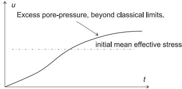
FIG. 11. The excess pore pressure recorded during wave-flume experiments by KIRCA *et al.* [11].
