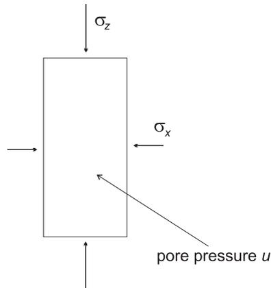
FIG. 12. A sample investigated in the triaxial apparatus.
