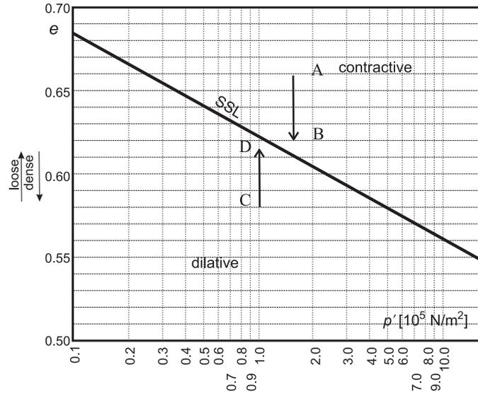
FIG. 2. The steady state line and initially contractive and dilative states of granular soil.
