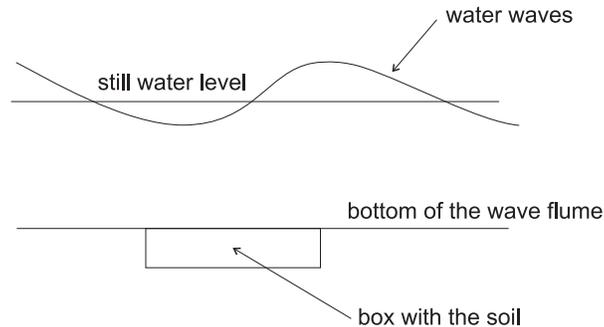
FIG. 10. A scheme of experiments, dealing with pore-pressure changes caused by water-waves, after [11]. Pore-pressure gauges were installed in the box.
