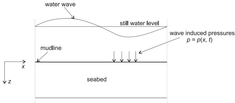
FIG. 3. Water waves induce cyclic changes of pressure at the mudline.
