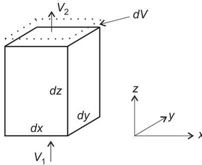
FIG. 8. 1D elementary volume of saturated soil.
