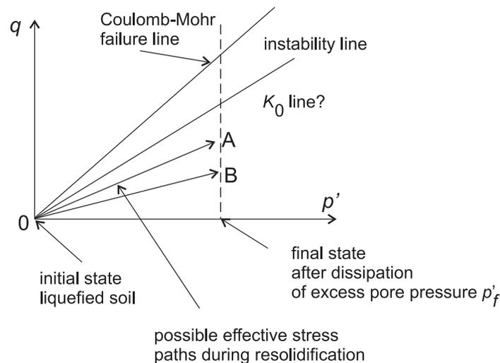
FIG. 7. Possible effective stress paths during the resolidification of liquefied soil.
