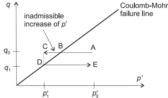
FIG. 4. Regrouping of effective stresses under wave-induced pore pressures.
