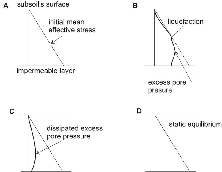
FIG. 5. Sequence of events from liquefaction to the dissipation of excess pore pressure.
